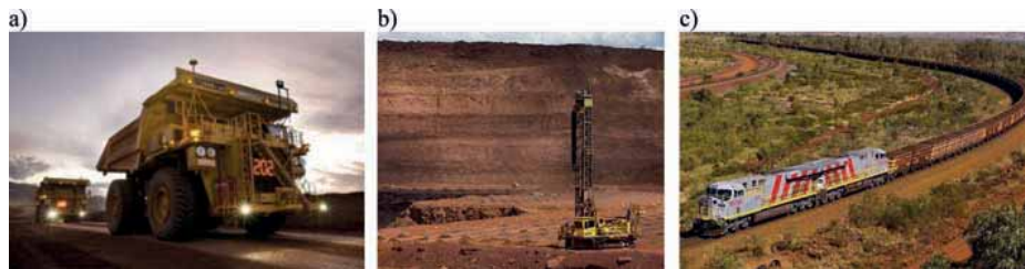
Figure 2. Exemplary autonomous heavy equipment used in iron ore mine in West Australia, Pilbara region.
