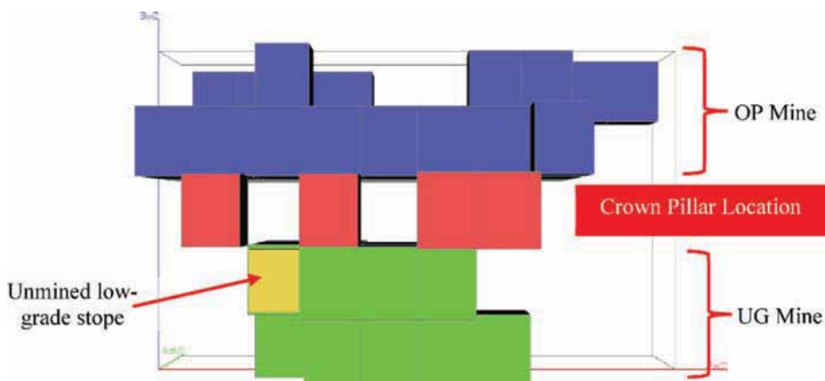
Figure 4. A sectional view through the block model showing the open pit limit, crown pillar and underground mining regions for the case study.
