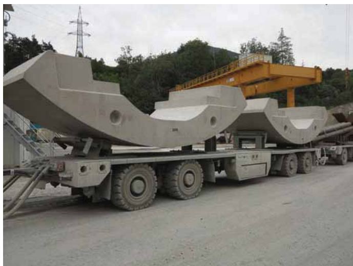
Figure 3. Four axle car loaded with pre cast concrete elements.
