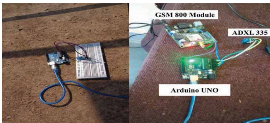
Figure 5. Integration of ADXL 335 accelerometer with Arduino microcontroller board and GSM.
