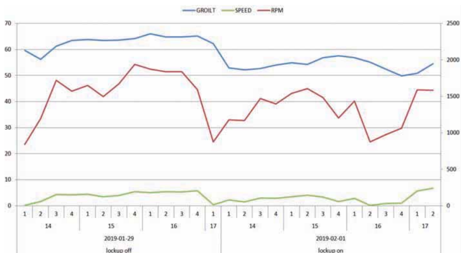
Figure 8. Influence of lock up system on oil temperature.
