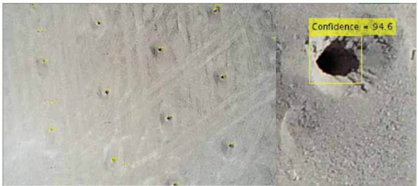
Figure 5. Drillholes detected using an image captured at 60 ft (18.3 m) AGL including confidence percentage.
