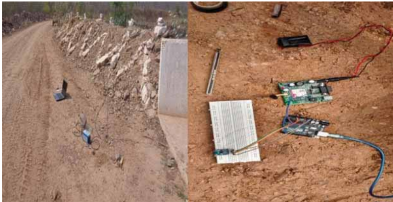
Figure 6. Installation of test bed in Mine-A.
