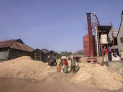
Recirculating dryer fuelled by shelled maize cobs.
