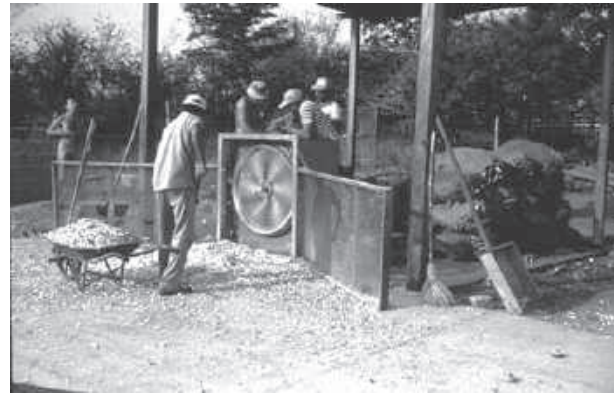
Figure 21-5. Cassava chipping machine in operation, using a "Thailand" type disk.
