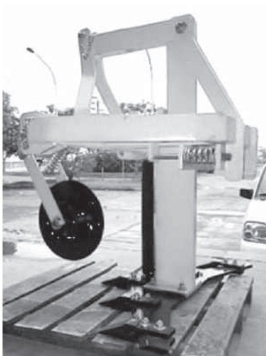
Figure 20-19. Prototype of a cassava harvester, model P 900 Flexible.
