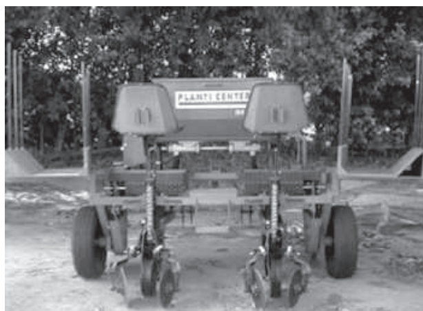
Figure 20-13. The modified 2-furrow cassava planter, Planti Center model Bazuca 1.
