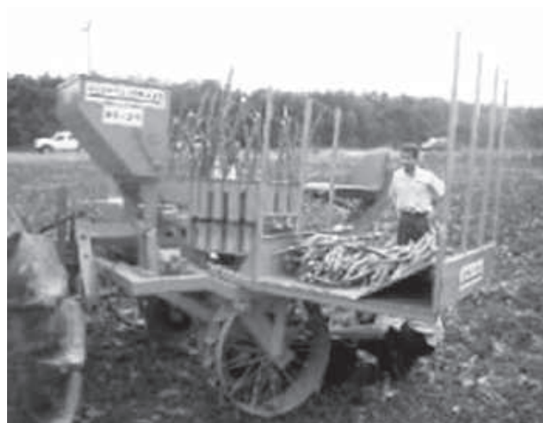
Figure 20-8. Two-furrow cassava planter, model PC-20.
