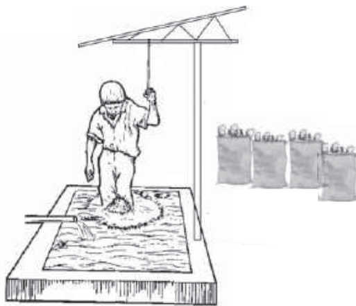
Figure 26-8. The roots are peeled by the feet during the washing operation in some cassava starch extraction plants. Friction causes the bark to come off.
