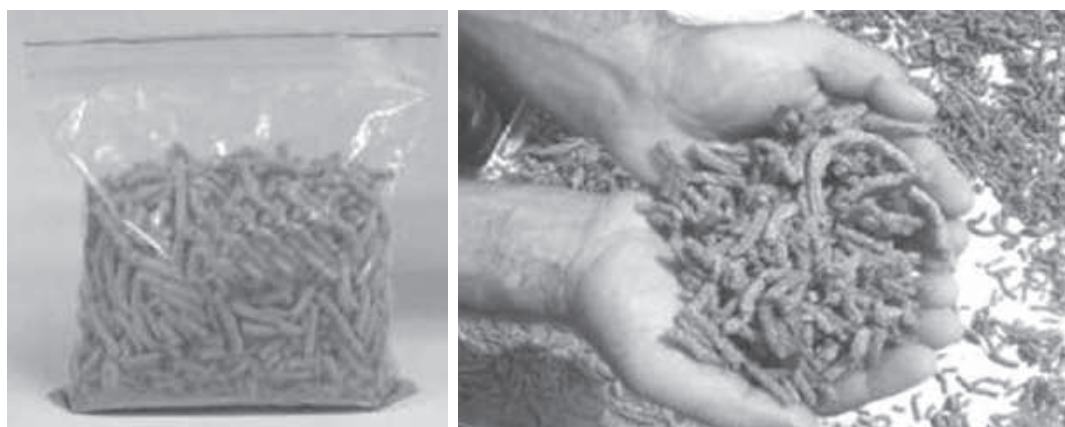
Figure 24-11. Final appearance of the organo-mineral fertilizer produced from crop wastes and vinasse produced during the processing of cassava into bioethanol.
