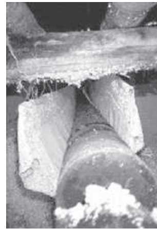
Photo 26A-3. Continuous sieving of the grated cassava using a worm screw.
