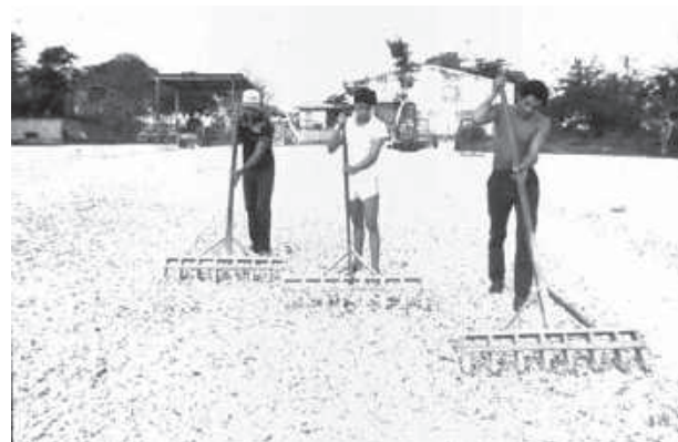
Figure 21-7. Cassava chips are turned over every 2 hours, using wooden rakes. The rakes may be constructed at the plant itself, especially for this task.
